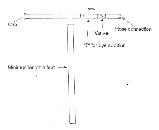
To be constructed of 3/4 or 1 Inch rigid steel pipe
